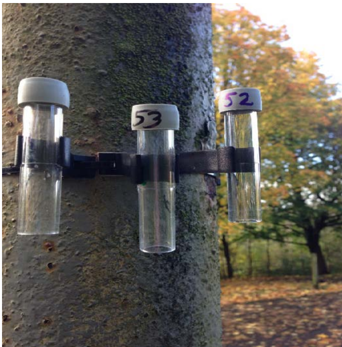
Figure 4 and 5: deployment of tubes
